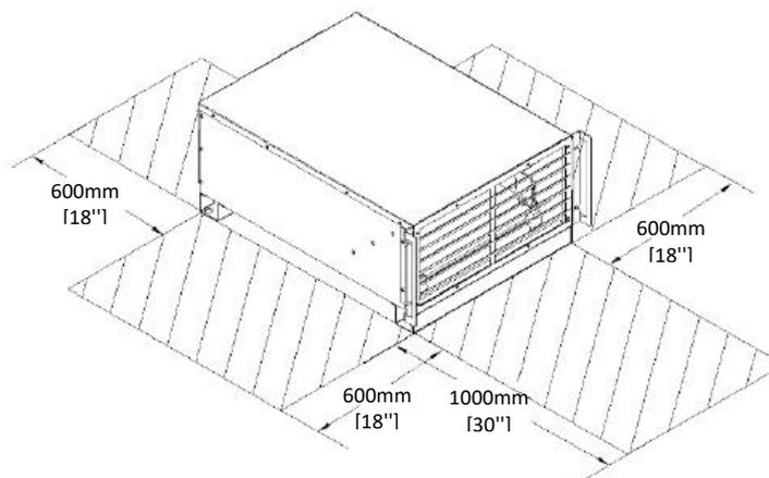
**Figure 2-9 Minimum Distance for Pull-out during Maintenance (Top View)**
