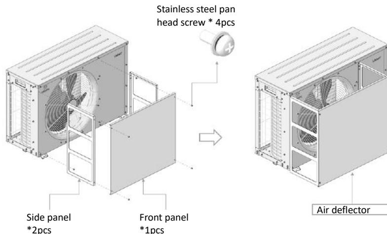
**Figure 3-21 Air Deflector Installation for Standard Condensing Unit**
