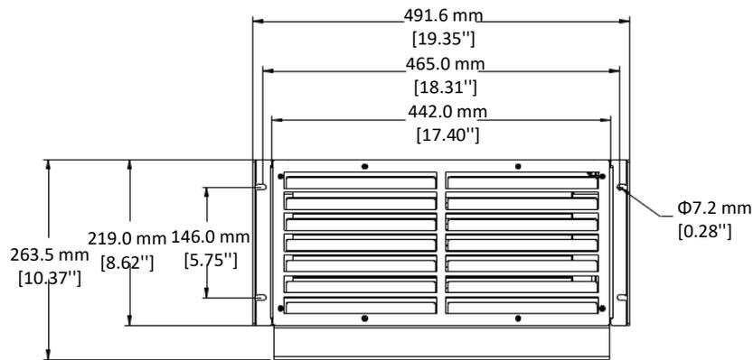
**Figure 3-6 Front View of Indoor Unit**
