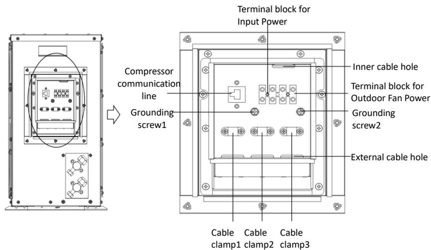
**Figure 4-6 Standard Condensing Unit Electric Connection Illustration**
