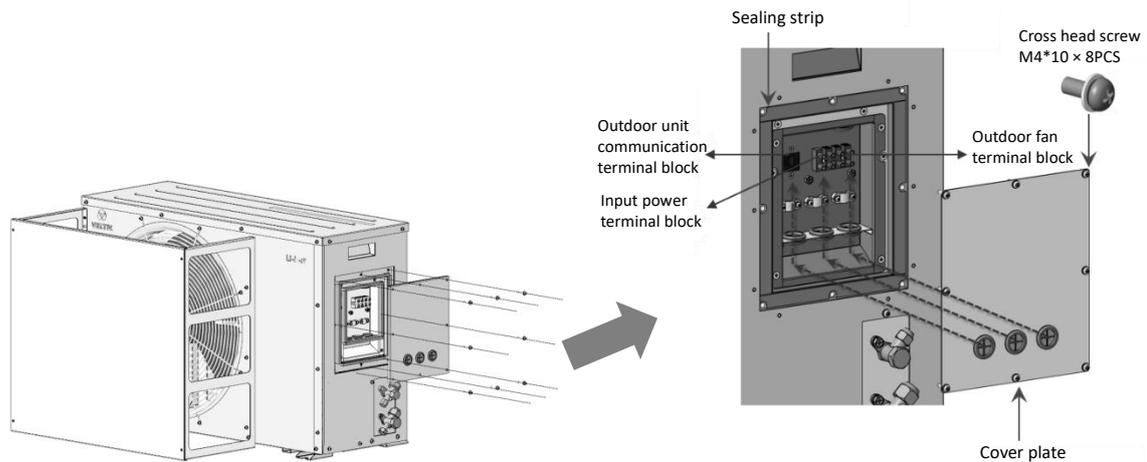
**Figure 4-5 Input Cabling Connections – Condensing Power Terminal**
