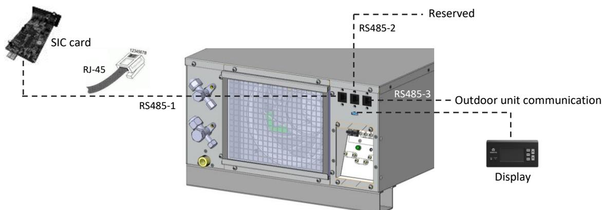
Figure 4-8 Communication and Monitoring Cable Connections in the Indoor Unit
