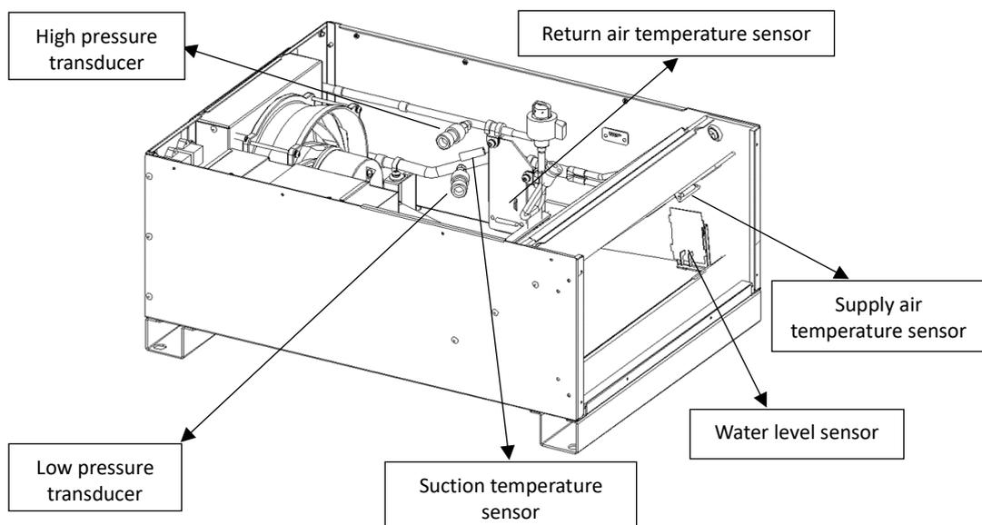
**Figure 1-6 Indoor Unit Sensor Location**
