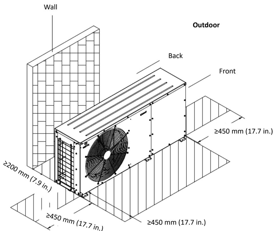
**Figure 2-13 Recommended Clearance Space Required for Low Ambient Condensing Unit**
