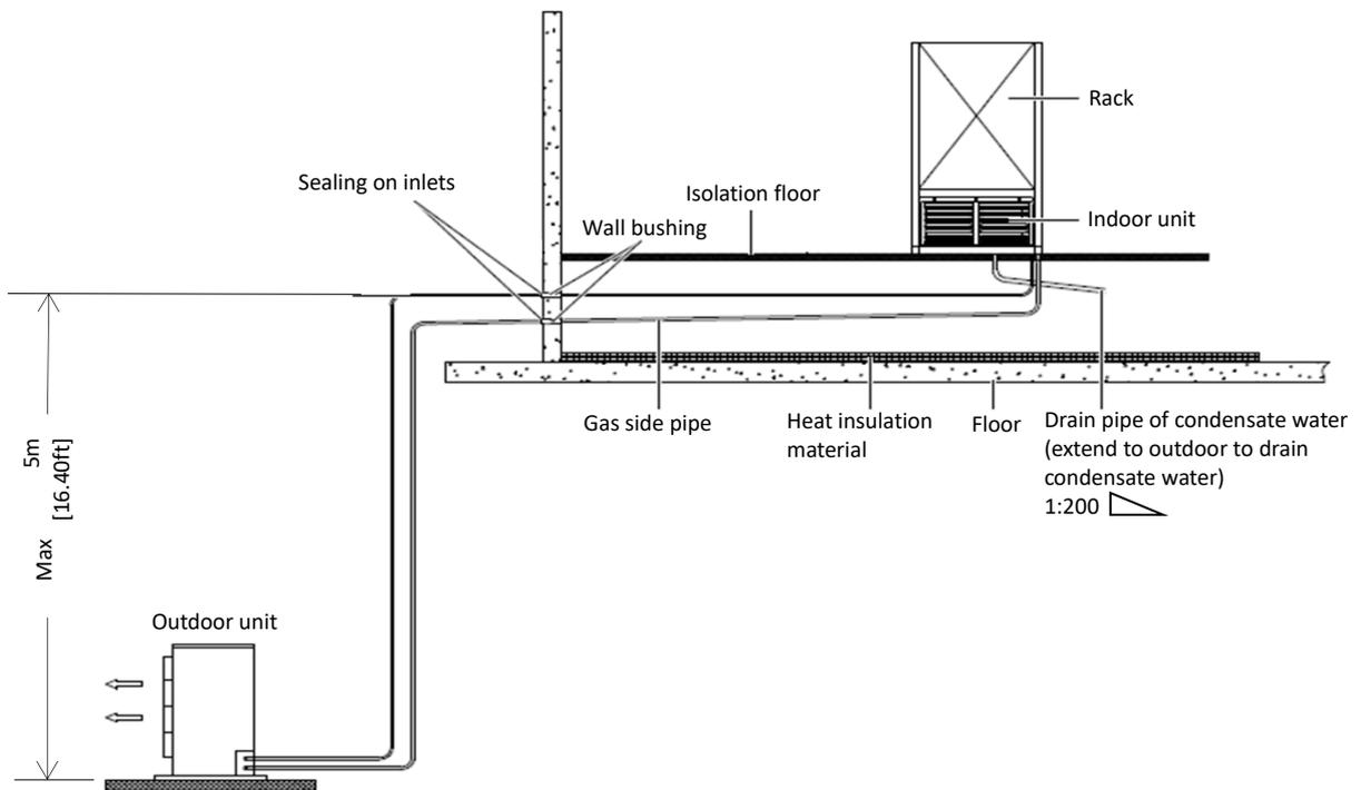
**Figure 3-12 Condensing Unit Installed Lower Than the Indoor Unit**
