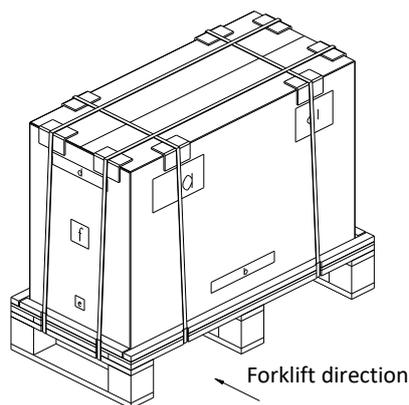
**Figure 2-5 Forklift Direction**
