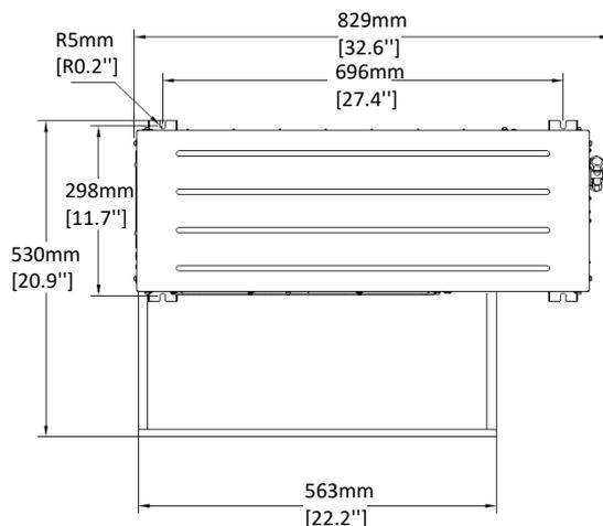
**Figure 3-9 Standard Condensing Unit Top View**
