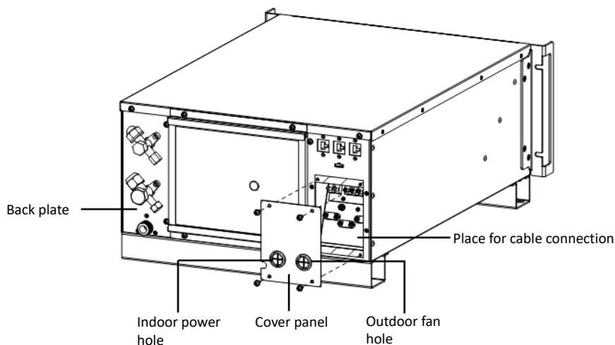
**Figure 4-1 Cover Panel for Cabling Connections**
