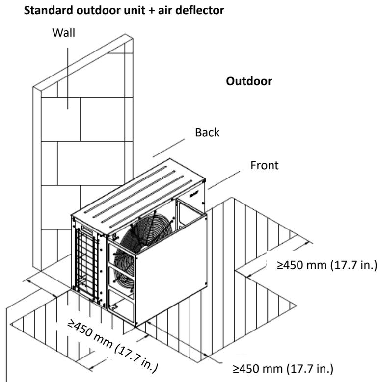
**Figure 2-12 Clearance Space Required for Standard Condensing Unit With Air Deflector**
