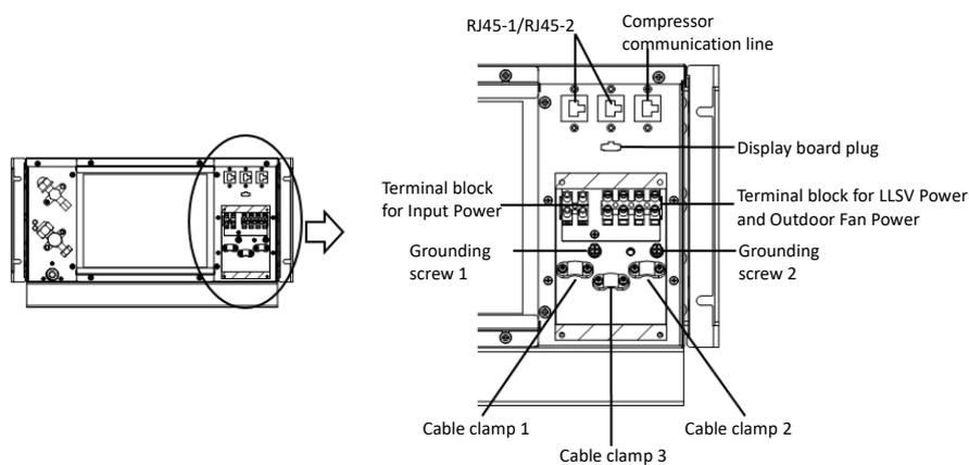
**Figure 4-4 Input Cabling Connections – Indoor Power Terminal**
