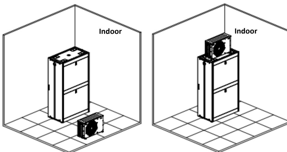
**Figure 2-10 Standard Condensing Unit Without Air Deflector for Indoor Use**
