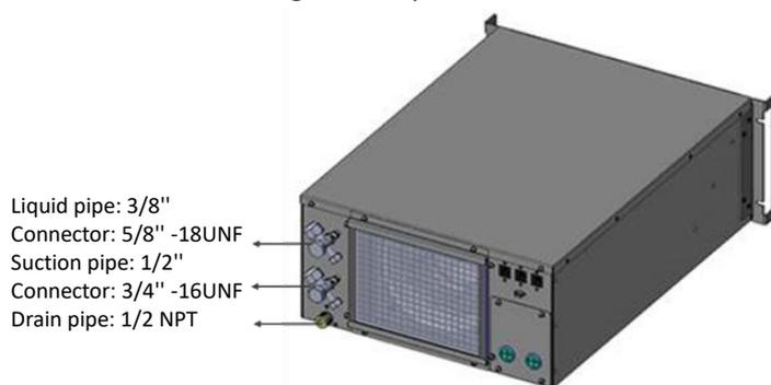
**Figure 3-22 Connectors of Indoor Unit**
