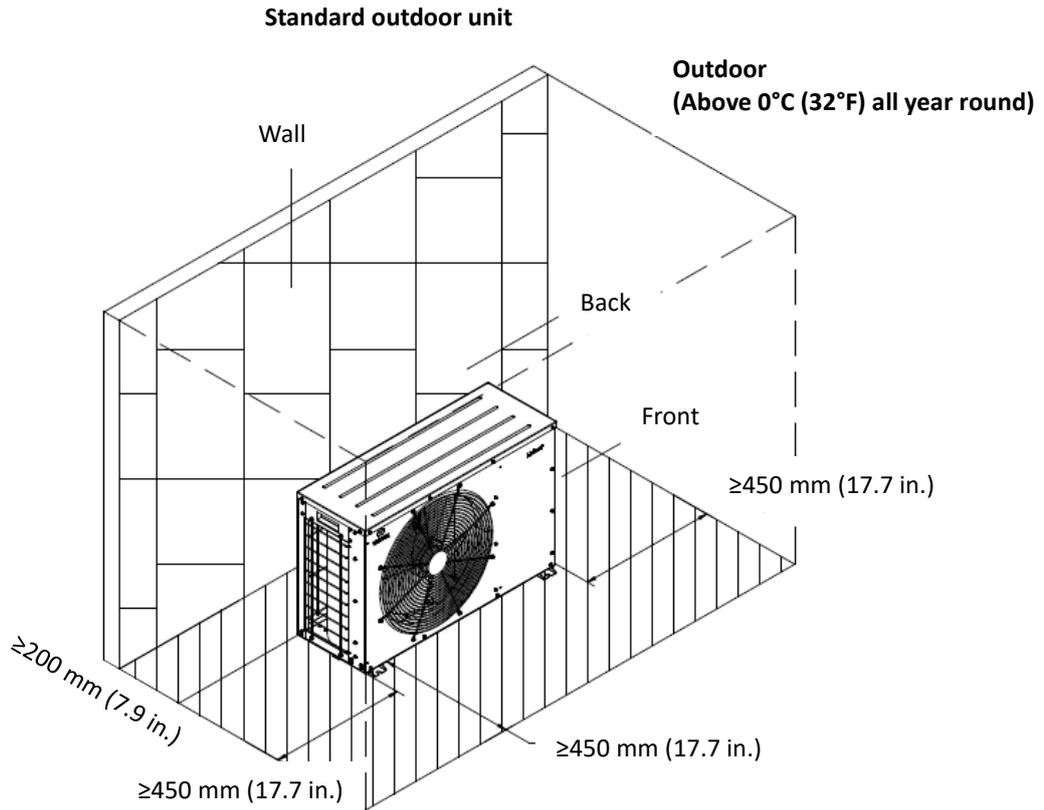
**Figure 2-11 Clearance space required for standard condensing unit without air deflector for outdoor use**
