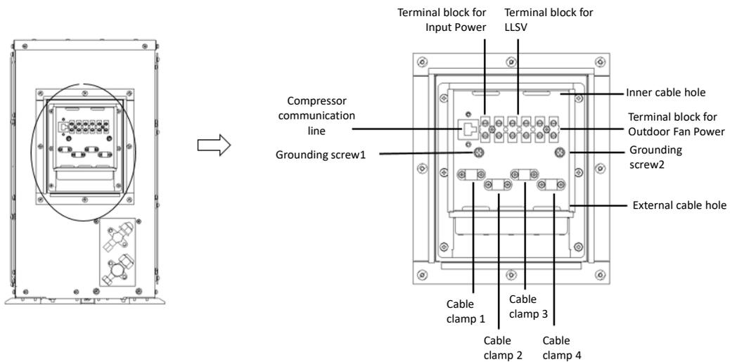
**Figure 4-7 Low Ambient Condensing Unit Electric Connection Illustration**
