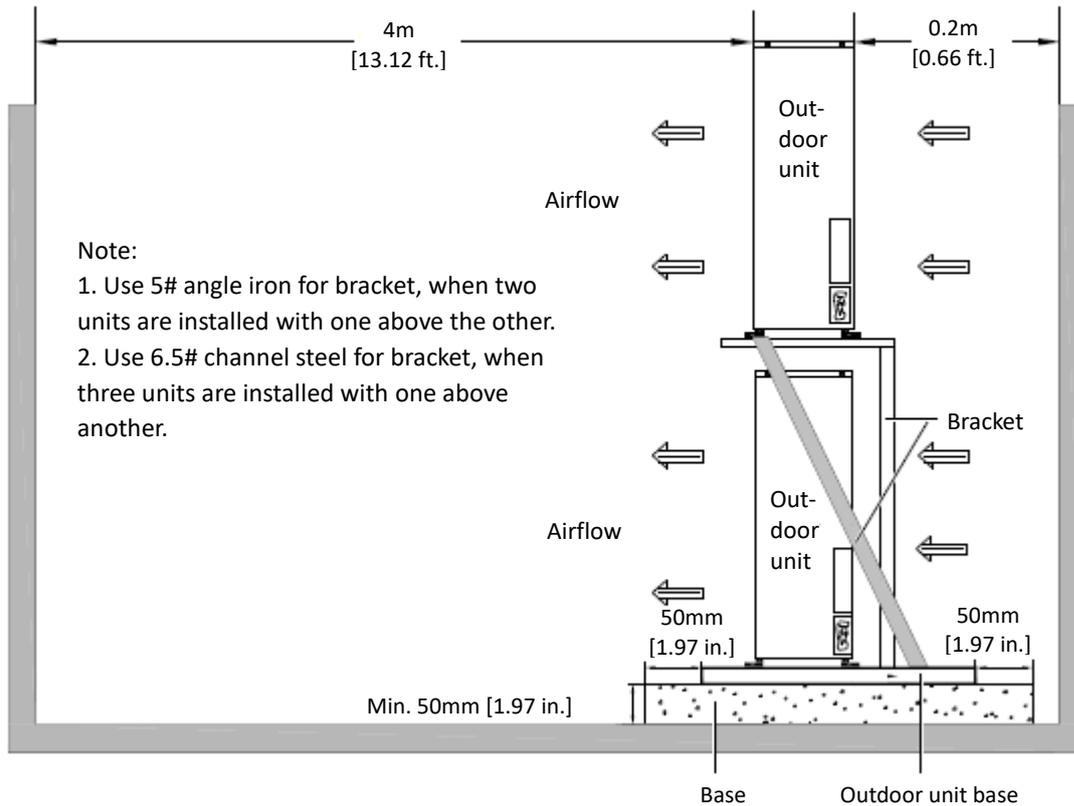
**Figure 3-13 Installing Multiple Condensing Units with One Above the Other**
