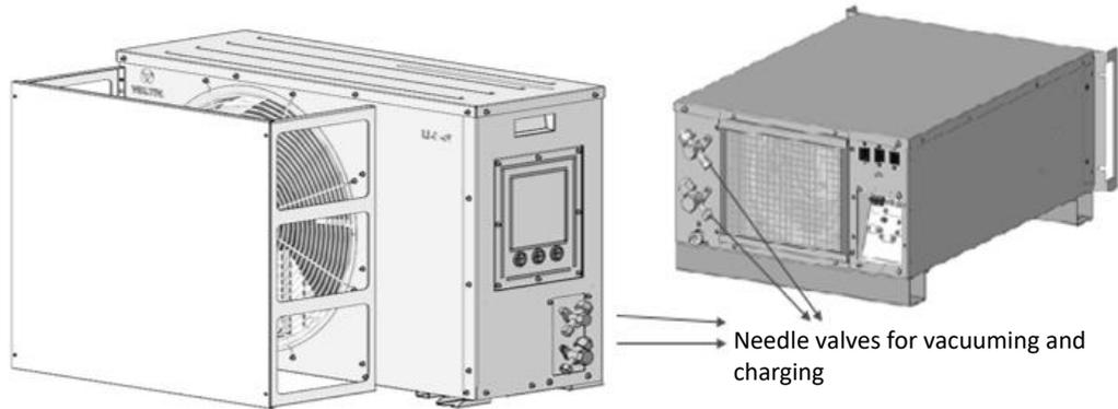
**Figure 3-27 Charging the Refrigerant Gas**
