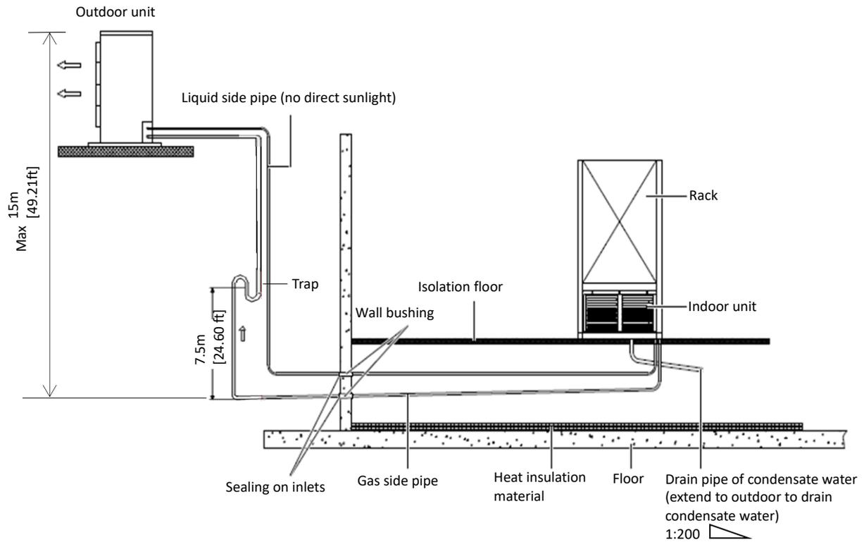
**Figure 3-11 Condensing Unit Installed Higher Than the Indoor Unit**
