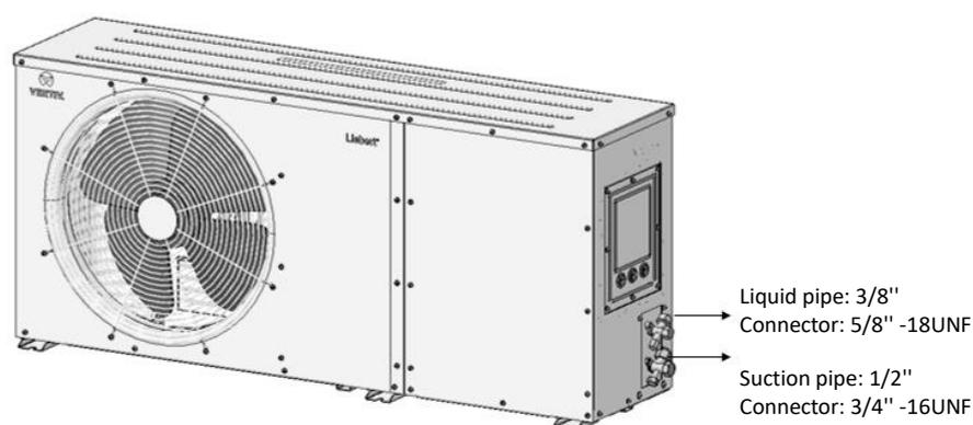
**Figure 3-24 Connectors of Low Ambient Condensing Unit**
