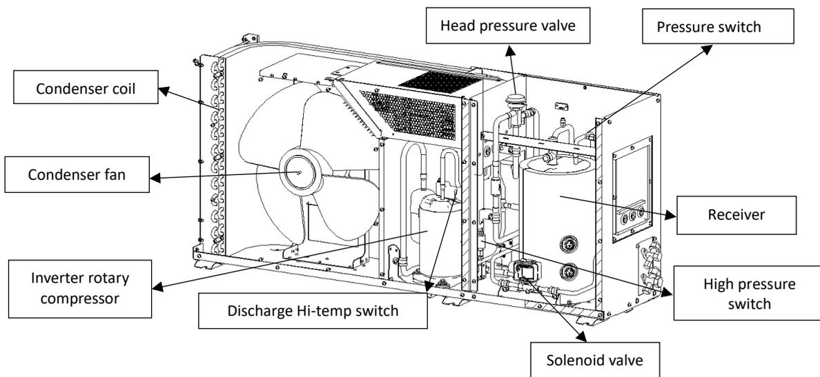
**Figure 1-8 Low Ambient Condensing Unit Internal Parts**
