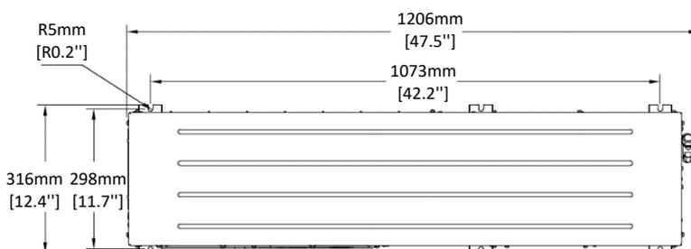
**Figure 3-10 Low Ambient Condensing Unit Top View**
