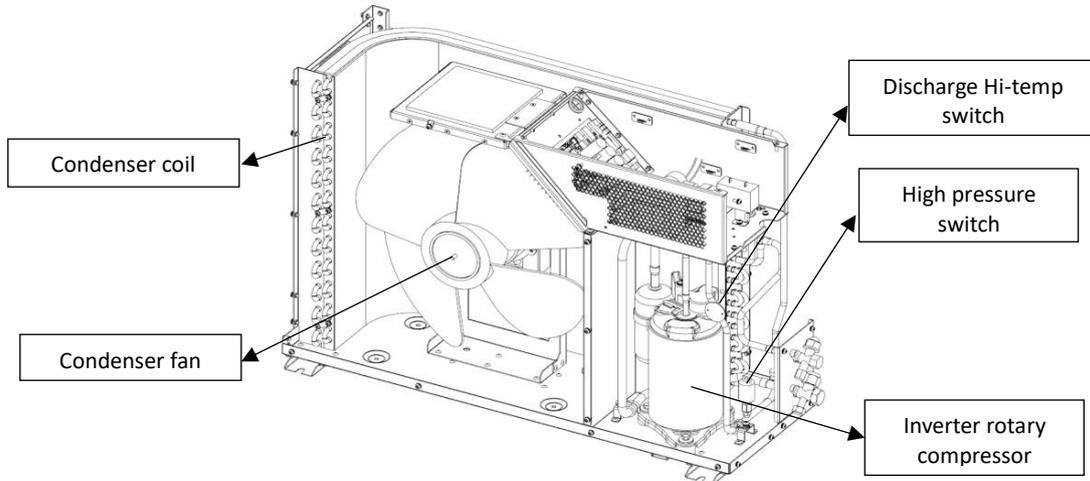
**Figure 1-7 Standard Condensing Unit Internal Parts**
