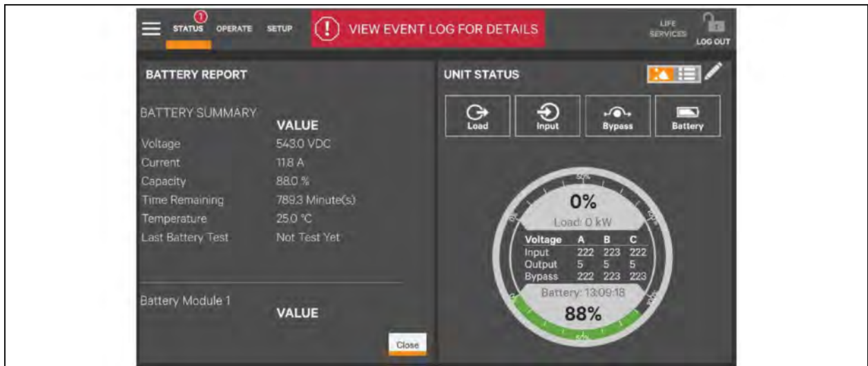
Figure 5.5 Battery Report—Unit Status
